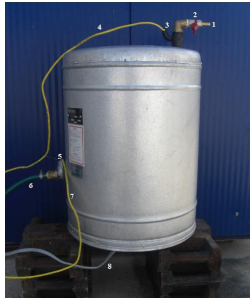
Fig. 2 Tank with PCM equipped with thermocouples to measure temperature
